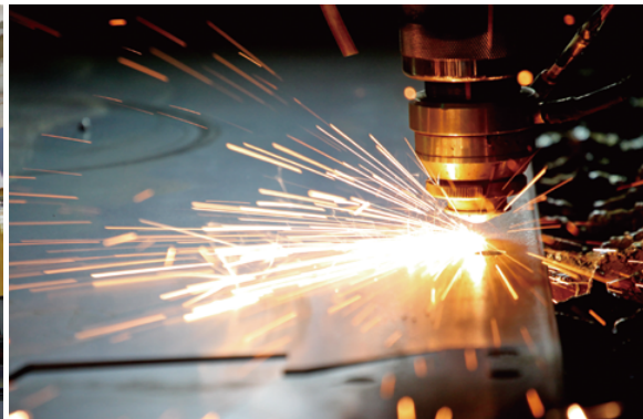
激光切割 Laser cutting
